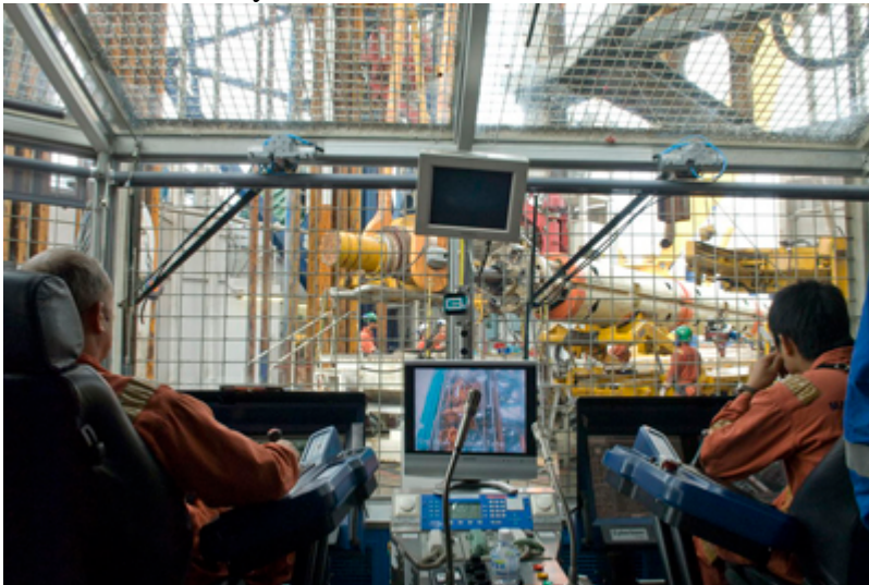
2- Disassembling riser pipes (view from the "dog house")
